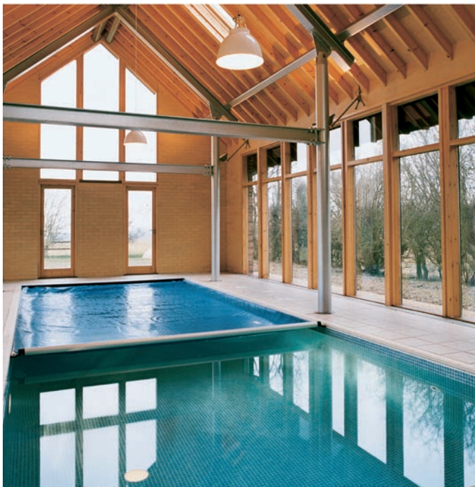
For indoor pools, a cover provides the added benefit of eliminating the need for expensive dehumidification systems.
