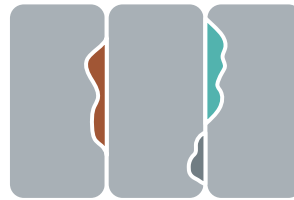
Galvanic corrosion occurs when different metals touch
