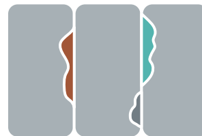
Galvanic corrosion occurs when different metals touch
