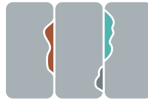
Galvanic corrosion occurs when different metals touch
